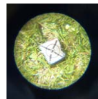
Rotate plummet 90° to check centring
